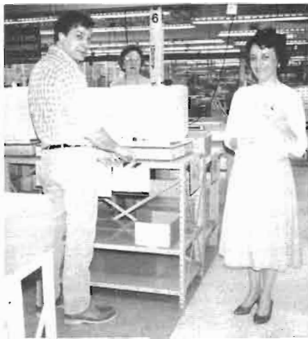
John deposits the production cards into the bin to reflect the completion of the Alpha unit. This alerts QC test that these units are ready to be pulled to the next unit.
