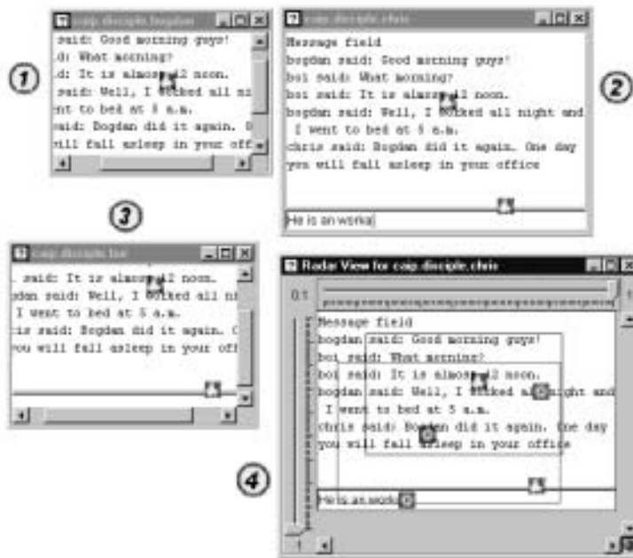
FIGURE 3 Collaboration widgets. Three users, bogdan (1), chris (2), and boi (3), collaborate over a chat bean and also post notes. User chris can see in his radar view (4) a view of the bean, the notes, telepointers, and viewing areas of all the users.
