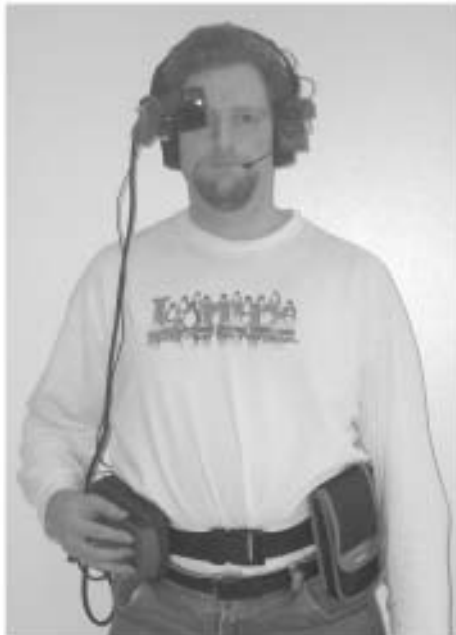
FIGURE 6 The Xybernaut MA IV wearable computer used in collaborative experiments with DISCIPLE.
