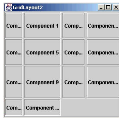
Figure 9. Resize 14 multisized labels using a GridLayout2 layout manager
