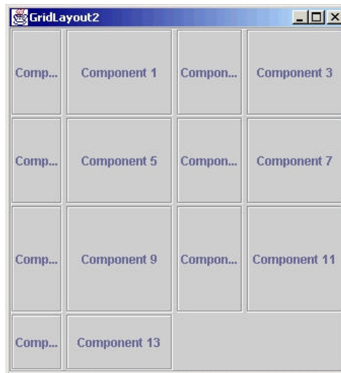
Figure 3. Arrange the same 14 labels with GridLayout2 layout manager
