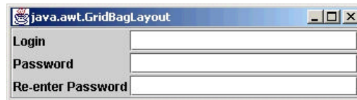
Figure 5. Sample change-password panel using GridBagLayout layout manager
