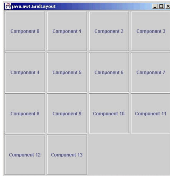
Figure 1. Arrange 14 multisized JLabels with GridLayout layout manager
