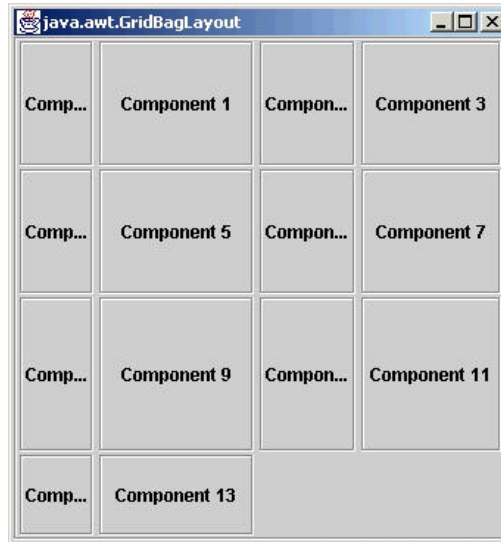
Figure 2. Arrange 14 multisized JLabels with GridBagLayout layout manager
