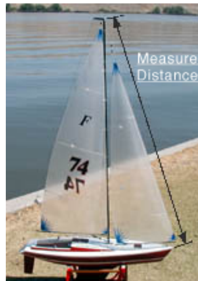
Figure 4. Measure Rake of Mast
