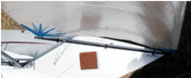
Figure 6. Camber in the Jib Sail
