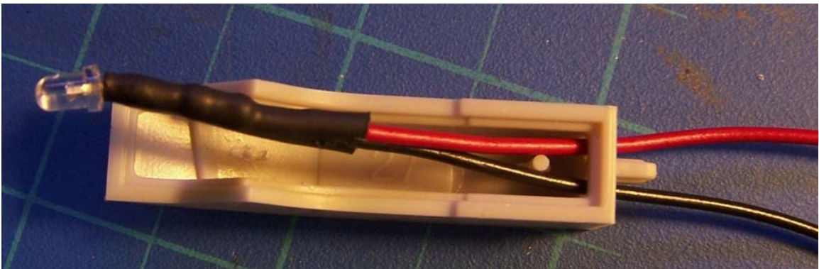
LED mounted in landing bay arm.
