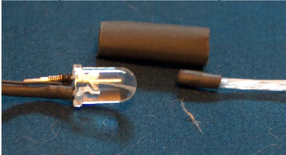
Fig 1, joining LED to fibers with heatshrink.
