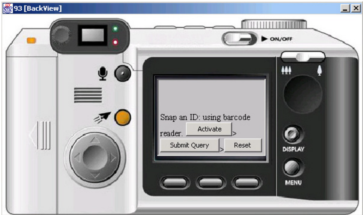
Figure 4. Screenshot of the back of a simulated bar-code-reading camera equipped with a miniature web browser.
