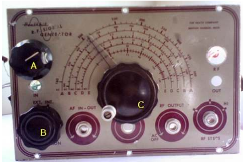
A is regeneration; B is RF attenuator and power; and C is tuning.
