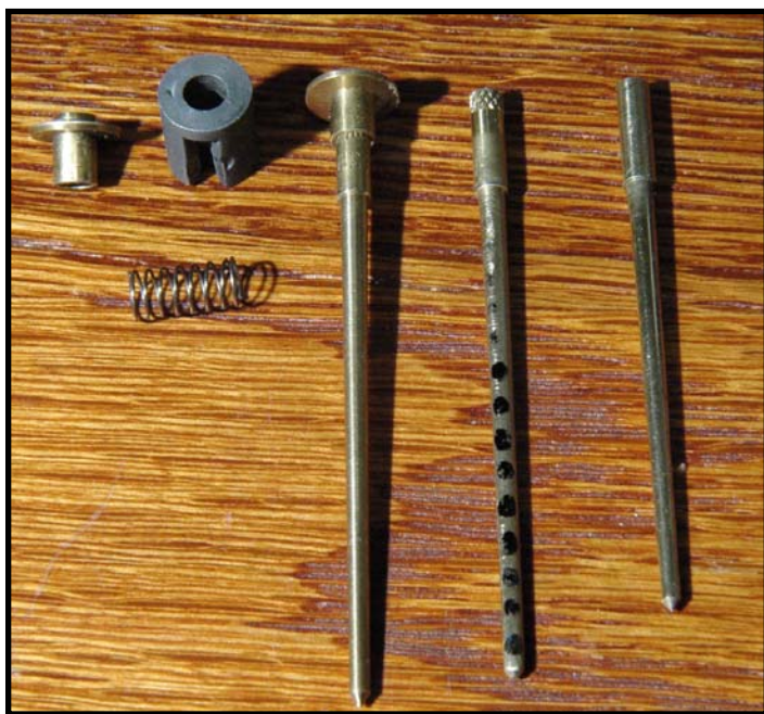
Photo 1) Various SU carburetor needles and other needle attachments. From the left: The biased collar attachment removed from a biased needle. The bushing that loosely holds the biased needle. The spring that gives the biased needle its spring action. A biased needle with the collar in place. A biased needle with the collar removed (note the knurled top to retain the collar). A fixed-type needle.
